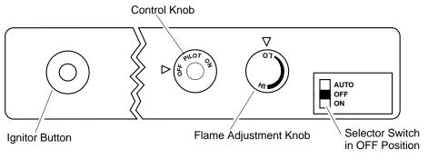
Figure 21 - Control Knob and Ignitor Button Location
